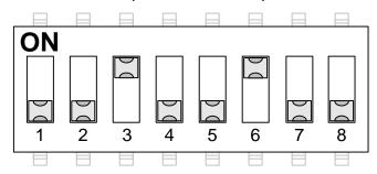
DCE (Pin 4 DSR Input and Pin 6 DTR Output)
